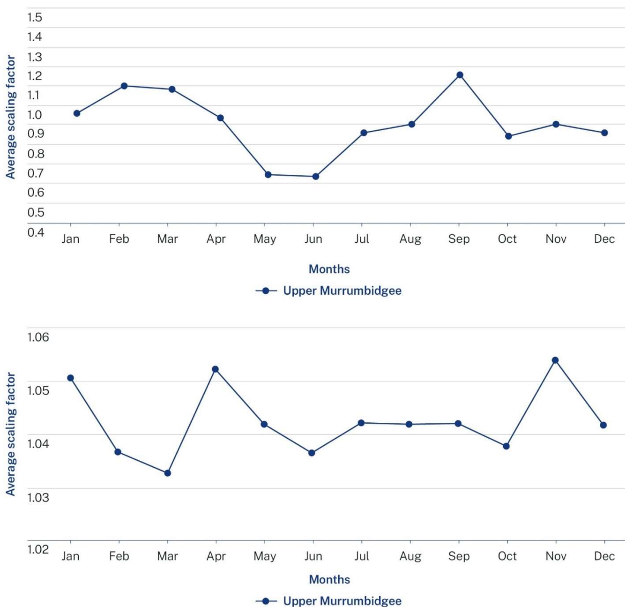
Figure 12. Average monthly changes in rainfall (top) and potential evapotranspiration (bottom) for the Upper Murrumbidgee under the dry future climate scenario for 2060–2079 compared to 1990–2009
